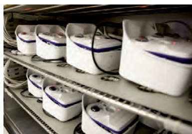
Each camera is tested at extreme temperatures before shipping.
