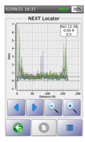
TestPro offers fault location for Return Loss, NEXT, and Shield aiding in problem identification. Support for MPTL, Patch Cord, Single Pair, GG45, Tera, and Coax is available through hot swappable adapters. At the completion of the Autotest, you get a highly visible Pass or Fail indication, and test results can be automatically saved with a customizable labeling scheme.
