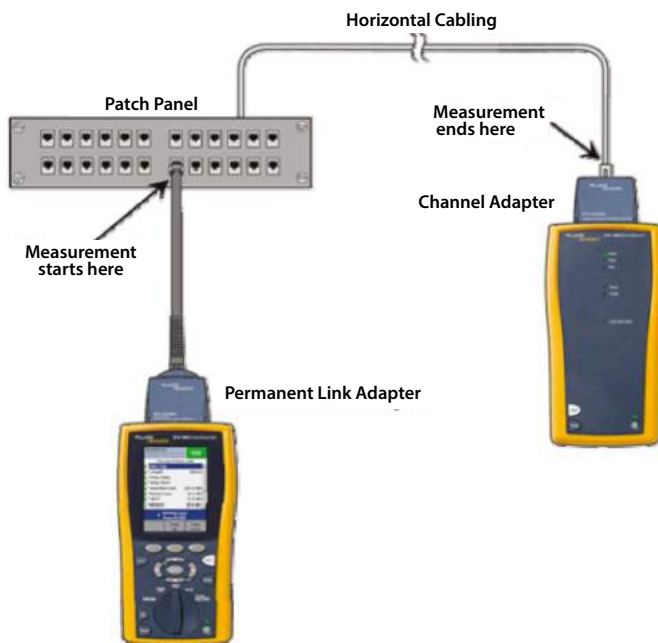
* Remote channel adapter & RJ45 plug are excluded from the measurement using Digital Signal Processing
