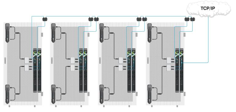
The PDU's can be daisy chained together to create a series of intelligent networkable handles that can be opened locally or remotely through the free software.
