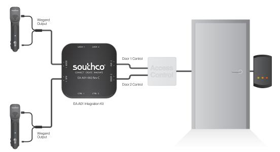
When integrated with an existing access control system, the new Integration Kit facilitates complete remote control and monitoring from building and room access down to server door access.
