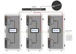
Each unit can support two locks, so both front & rear doors to a cabinet can be placed on a Sentry unit. Using PoE makes this an easy and cost effective application, which allows for integration into existing access control panels.
