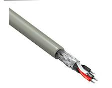
Aura multicore 7/0.2 overall screened cables are manufactured with stranded tinned copper conductors and have an overall screen and overall braid, with LSZF Sheath.
