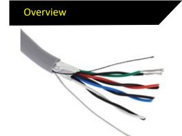
Aura multipair 7/0.2 screened cables are manufactured with stranded tinned copper conductors and have an overall screen, complete with a stranded drain wire.
