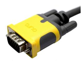
The Aura range of SVGA cables are a high-quality product, made using 26 AWG coaxial copper conductors with matching shielding and foil shield for main RGB colours. It also has 26 AWG conductors for the other pins with overall foil and tin copper braid providing a fully shielded 15 pin populated cable, . These VGA-SVGA Leads feature connectors robustly terminated connectors onto the cable with PVC insulation and support 1024 x 760 resolution.
