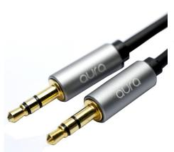
The Aura 3.5mm Jack Audio cables are a high quality fully shielded OFC copper cable product. These Premium 3.5mm Jack Audio cables are made using 28 AWG copper conductors with matching shielding ensuring good conductor abilities and very good protection against outside interference. Connectors are robustly terminated onto the cable with gold plated contacts minimising degradation in connection contacts. Insulation of the cables is a TPE outer sheath providing greater flexibility.
