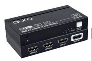
AR-40-110 is an HDMI 18Gbps 3x1 Switcher. It is an auto switcher with three HDMI video inputs and one HDMI output. It supports HDMI video resolution up to 4Kx2K at 60Hz 4:4:4 HDR, Dolby Vision and multichannel audio. It is powered by the HDMI input source and no need of any external power supply, is controlled by the IR remote and supports CEC pass-through.
