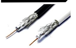
Aura MF100 is a 75ohm coaxial cable with 1.0mm Dia copper inner conductor, foam PE insulation, aluminium foil wrap, tinned copper braid and LSZH outer sheath both meeting Eca Standards. CAI Approved, Certificate CAI0157A
