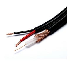
Aura RG59 Shotgun is a 750hm coaxial cable and 0.5mm or 0.75mm red/black Power cable for CCTV systems. Cable features 0.58mm Dia copper clad steel inner conductor, Solid PE insulation, copper clad aluminium braid and PVC or LSZH outer sheath both meeting Eca standard. Also features red and black insulated stranded copper power conductors in overall PVC/LSZH outer sheath.
