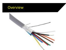
Aura multicore 7/0.2 screened cables are manufactured with stranded tinned copper conductors and have an overall screen, complete with a stranded drain wire.
