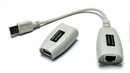
This Aura product extends USB 2.0 signal between Transmitter and Receiver over twisted pair CATx cable. It supports USB 2.0 signals up to 50M and does not require any power. The transmitter and receiver have short fly leads on each, the receiver being female USB, so a short male to male lead will be required for the final connection.
