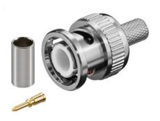
Male RG59 BNC Crimp connector. RG59 male BNC connector is supplied as the connector body, centre pin and crimping collar and is only suitable for RG59 75ohm Coaxial cable. Installation of the connector must be carried out with the correct stripping and crimping tools, pack of 10.
